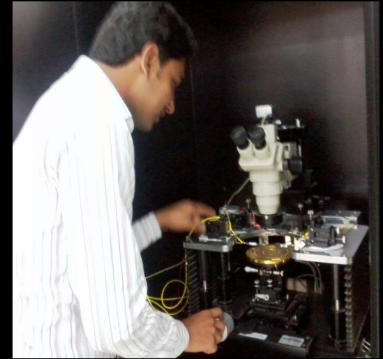
IC Testing using Probe Station
